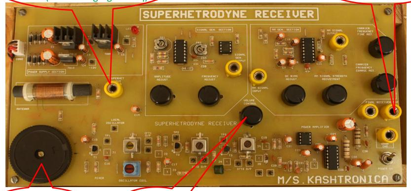
Adjust tuning control so as to get maximum output voltage sinusoidal signal on DSO
